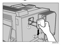
When installation is complete, the printer hard disk is automatically formatted.
