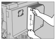
Install the printer hard disk on the back of the controller board.
