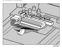
Align the controller board with the top and bottom rails, and then slowly push it in until it stops.
