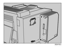
Use a coin to fasten the screws securely.
