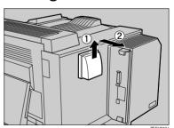
A Remove the other dustproof filter cartridge by lifting it up.
