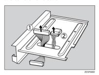
Connect the flat cable (1) and power cable (2) to the printer hard disk.
