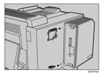
The removed screws are used in step **(1)** to refasten the controller board.
