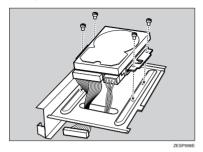
Use a coin to fasten the screws tightly.
